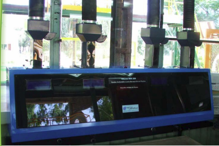
Multipoint device for analysing incoming grains
