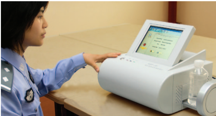
A water bottle is tested with the AY01-01 Rapid Liquid Contraband Detector, enabled by Ocean Optics' QE65000
