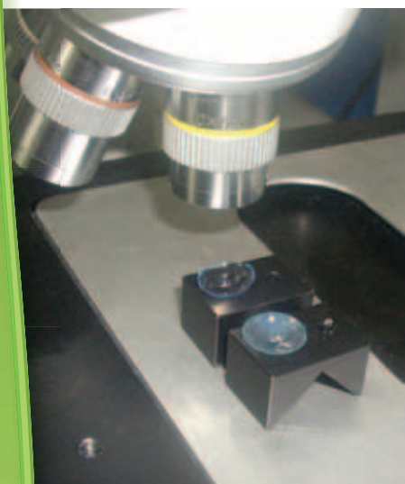
Silicone hydrogel lenses analysed with the NanoCalc-2000-UV/VIS
